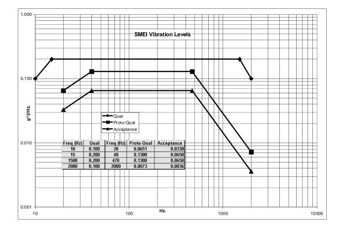
Figure 3.1 - Vibration Test Levels for SMEI (Acceptance Levels to be used for Flight Cameras)
