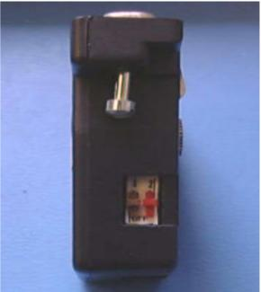
Figure 4. Write Enable And Watchdog Switches
