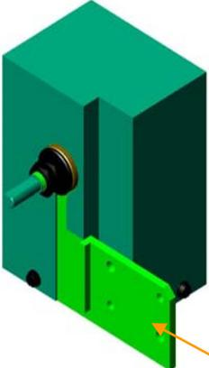
Mounting Interface to Structure Rear Panel
