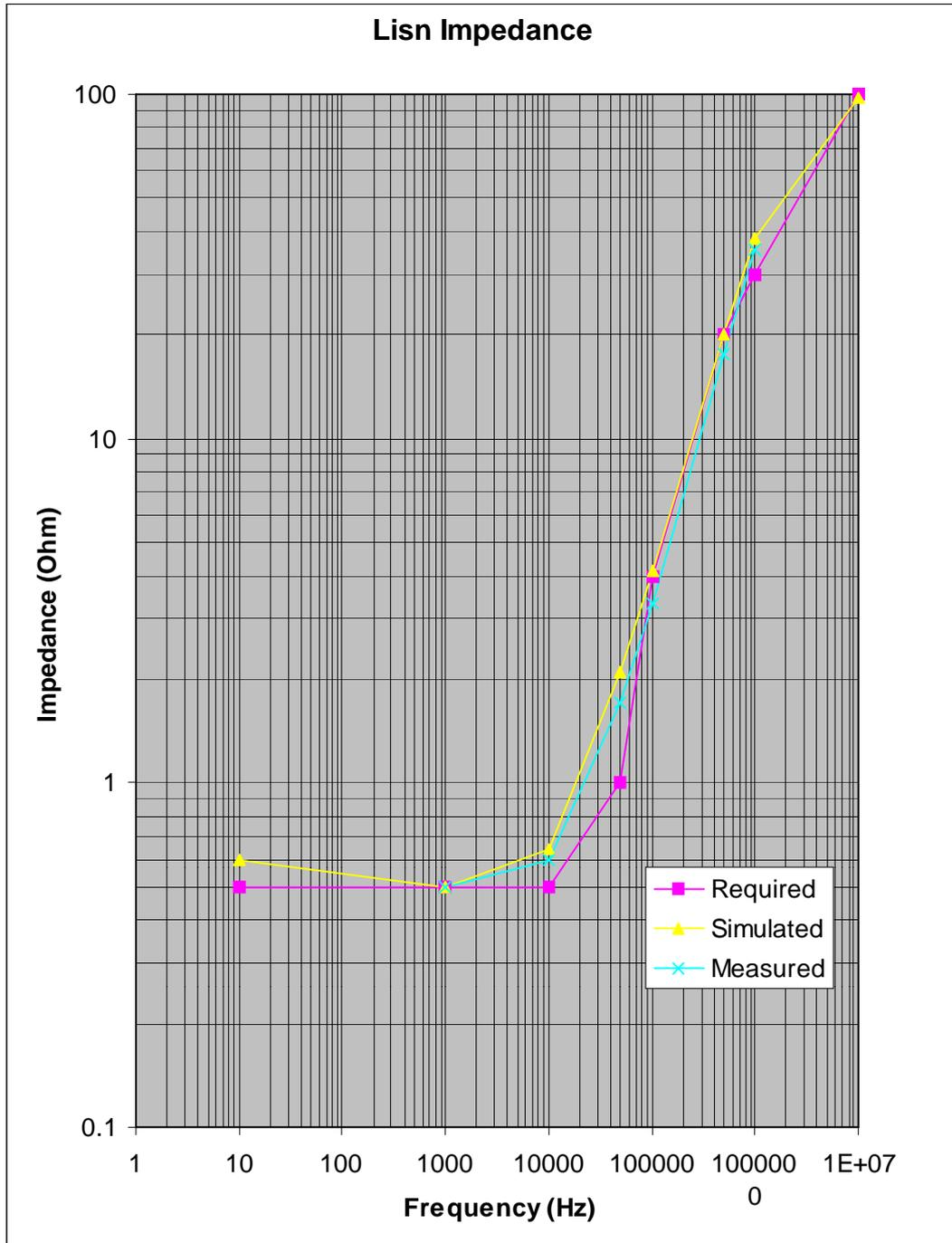
Figure A2 Magnitude Plot of LISN Impedance
