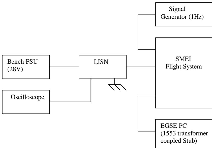
Figure 1 Ripple Measurement Test Setup
