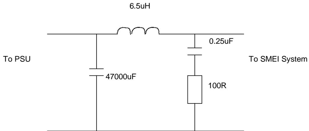
Figure A1 Simplified Schematic of the LISN
